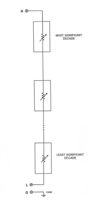
Figure 5.1. HPRS Series Schematic Diagram
